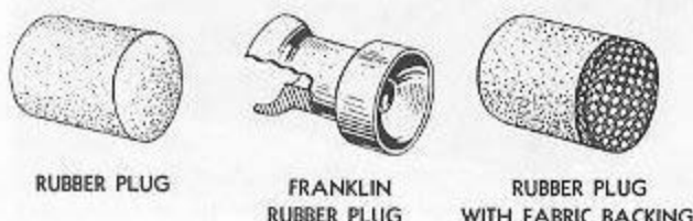
Figure 10-6.—Types of rubber plugs used for cleaning condenser tubes.
