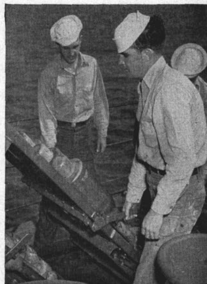
Official U. S. Navy photograph 'MOUSETRAP,' like the 'hedgehog,' is an 'ahead-thrown' weapon, in contrast with the earlier depth charge.
