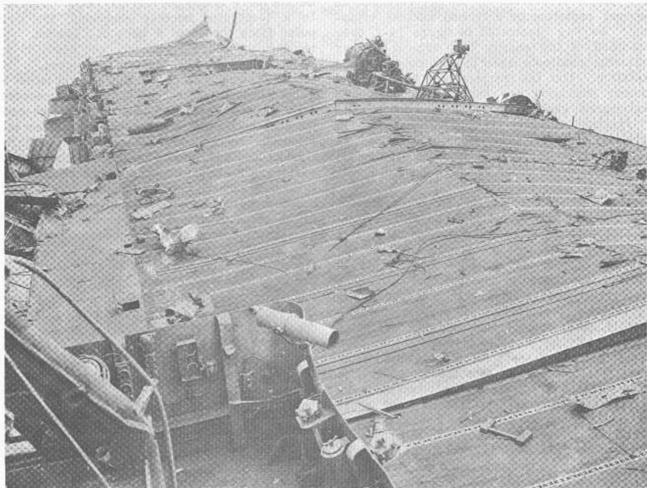
Figure 14-14.—Flight deck of carrier Independence after test at Bikini. Blast pressure entered the hangar deck from the side, through rupturing of side curtains. Flight deck was bulged upward whereas hangar deck below was dished downward.
